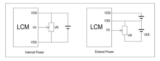
VDD-V0: LCD Driving Voltage
