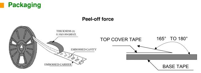
The peel off force of cover tape is 10 to 70 grams in the arrow direction.
