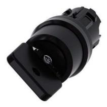
Key-operated switch O.M.R, 22 mm, round, plastic, lock number 73034, black, with 2 keys, 2 switch positions O-I, latching, actuating angle  $90^\circ, 10:30h/13:30h$ , key removal O, with laser labeling, inscription or symbol Customer-specific selection with SIRIUS ACT configurator (CIN)
