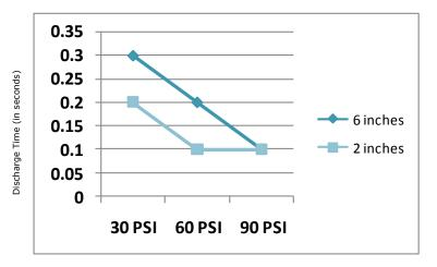
Offset voltage and discharge time per ANSI/ESD STM3.1 using a charged plate monitor with a 20pF, 6" x 6" plate. 1000 to 100 volts. Typical results.
