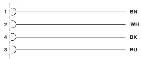
Contact assignment of M8 socket
