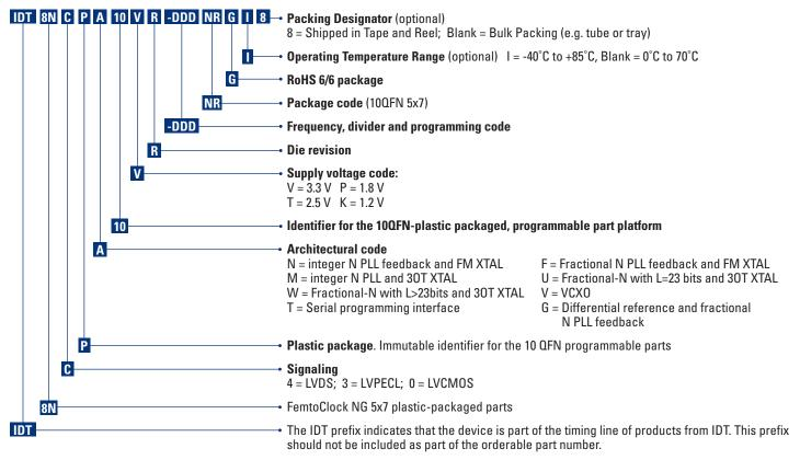
Example: IDT 8N3PN10VA-001NRGI8 is a LVPECL FemtoClockNG programmable clock generator with an internal integer-N feedback PLL, with the frequency coded by "001", 3.3 V, A-revision, in a RoHS 6/6 plastic 5x7 package (10QFN), industrial temperature and with tape and reel.
