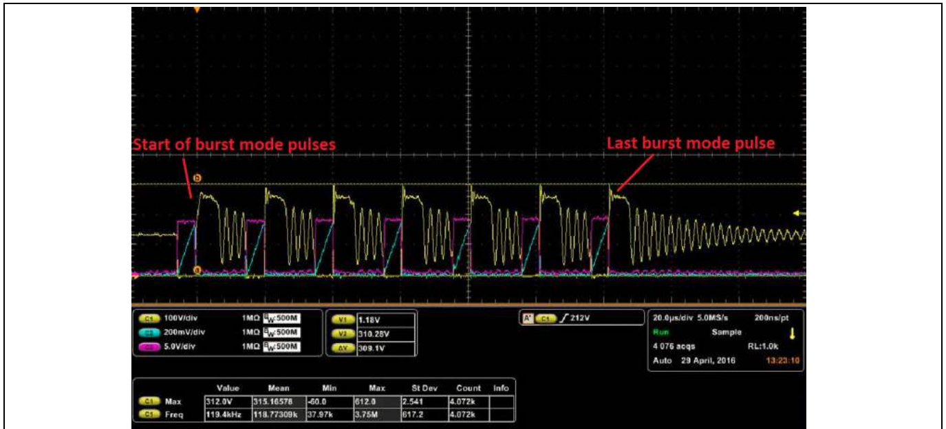
Figure 21 Low line (100 V AC ), no load, The ICE2QS03G is operating in burst mode to minimize the idle power consumption. The burst mode pulse train shown above occurs every 33.8 ms with the main switch inactive in the period between pulse trains to lower light load power consumption.
