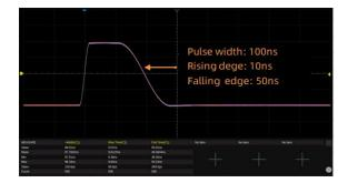
**Flexible edge** Adjustable fine step resolution to 100 ps. The minimum edge is 500 ps and can be generated at any frequency. The rising/ falling edge can be set respectively and can be used to generate asymmetric pulse
