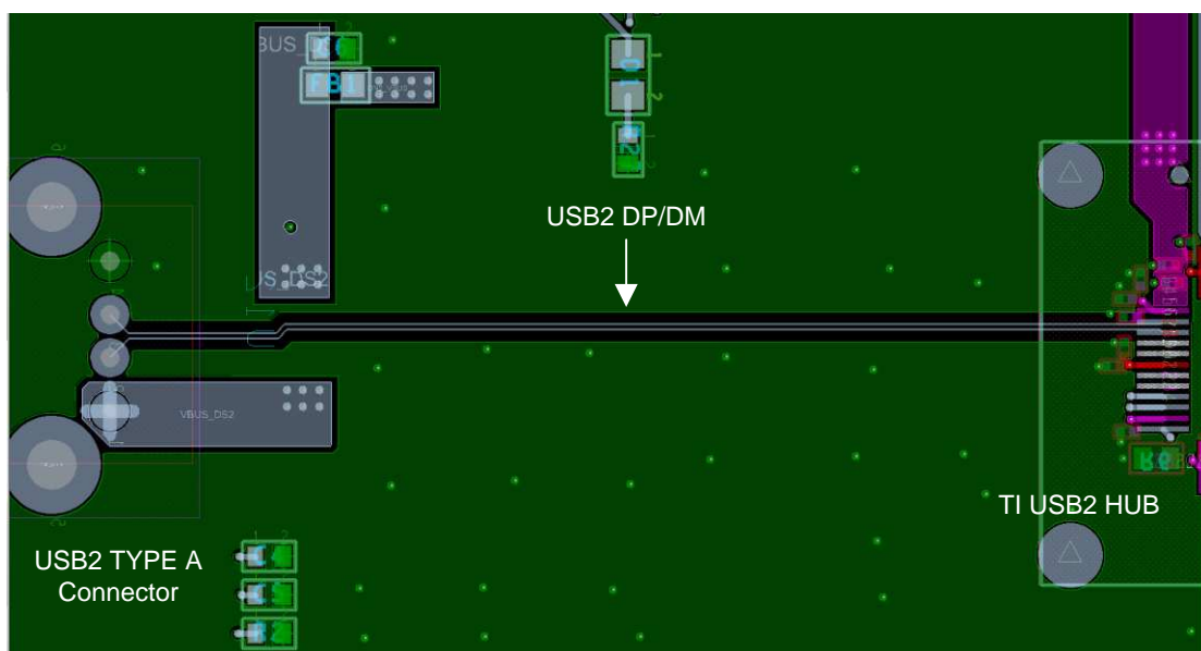
Figure 40. Example Routing of Downstream Port
