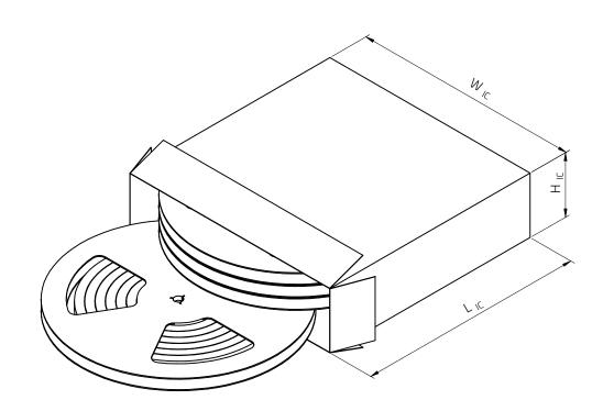
Packaging Specification - Carton: [mm] Т W No. of Qty. (pcs.) L<sub>C</sub> (mm) (mm) Material (mm) Inner Carton (pcs.) Tolerance typ. tvp typ. Value 360.00 360.00 400,00 Paper CHECKED REVISION DATE (YYYY-MM-DD) GENERAL TOLERANCE PROJECTION METHOD  $\oplus$ CHC 001.003 2022-10-20 DIN ISO 2768-1m DESCRIPTION **WE-CST Current Sense** Würth Elektronik eiSos GmbH & Co. KG **Transformer** ORDER CODE EMC & Inductive Solutions Max-Eyth-Str. 1 749252060 74638 Waldenburg
