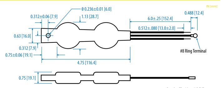
Leads: 6", stripped 0.51" Weight: 0.15 lbs/68g Gauge: 14 AWG
