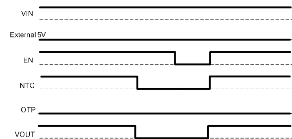
Figure 3: Normal Mode without external 5V \rightarrow NTC protection Mode \rightarrow EN Restart
