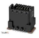
SMD male connector, nominal current: 1.7 A, Test voltage: 500 V AC, number of positions: 20, pitch: 0.8 mm, color: black, contact surface: Gold, contact connection type: Pin, mounting: SMD soldering
