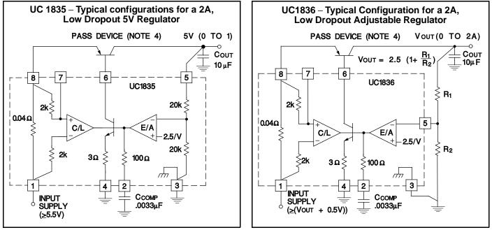
Note 4: Suggested Pass devices are TIP 32B. (Dropout Voltage ≤0.75V) or, D45H, (Dropout Voltage ≤0.5V), or equivalents.
