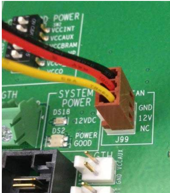
Figure 1-21: Heat Sink Fan Power Connector J99
