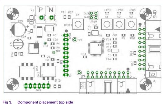
The upper left part of the board contains the KNX TP1 header K1 to connect the KNX bus. Below the KNX connector, the board contains the physical transceiver part of the design. On the left bottom side the isolated UART interface is available on header SV2.
