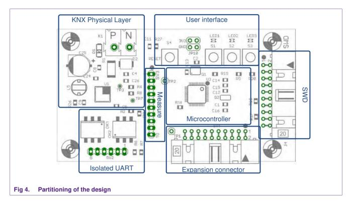
In the middle of the board, a header is available to measure the various signals between the microcontroller and the transceiver. The top part contains the user interaction: LEDs and buttons. The header on the right hand side provides a debug probe connection that complies with the Serial Wire Debug (SWD) interface standard. To interface with other boards an extension connector is present on the lower part of the board. See Fig 4.
