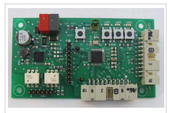
Fig 1. OM 13042 KNX TP1 NCN5120 LPC1227 evaluation board
