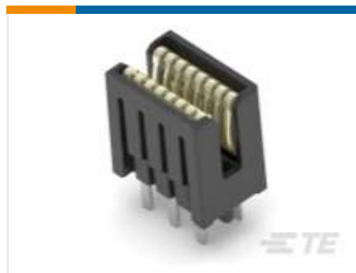
TE Part #2344604-1 50 AMP CARD EDGE ASSEMBLY
