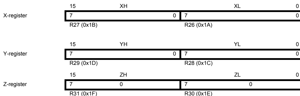
Figure 7-3. The X-, Y-, and Z-registers
