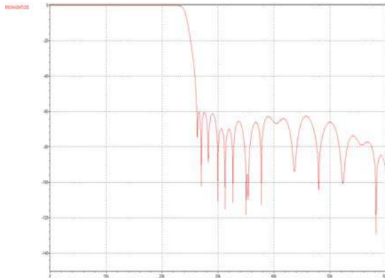
Figure 6 DMIC Digital Filter Frequency Response
