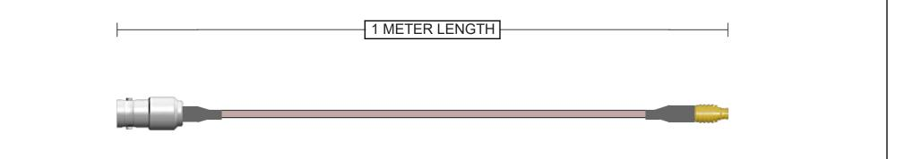
Connector A 112631 BNC Jack Straight Brass Nickel + Heatshrink 50 Ohm RG-178 Continuity/Hi-Pot Connector B SMP-FS-C19 SMP Plug Straight Beryllium Copper Gold + Heatshrink
