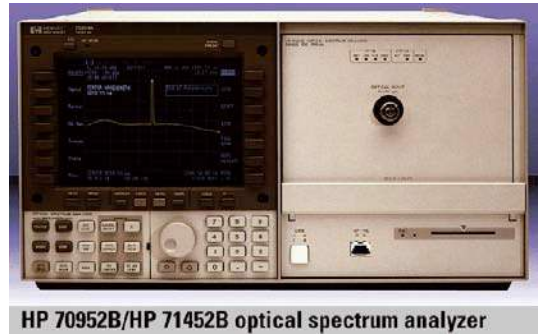
Photo 13. An optical spectrum analyzer is used to characterize the light outputs from LEDs and lasers.
