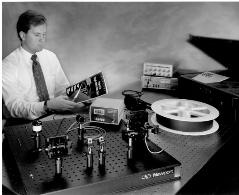
Photo 12. Engineer preparing to measure the attenuation through a spool of optical fiber. (Photo furnished by Newport Corporation.)
