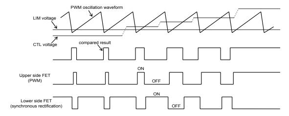
If a minus voltage is applied to the CTL pin, this pin current must be limited within 2mA by inserting the resistor of about  $200\Omega$ .
