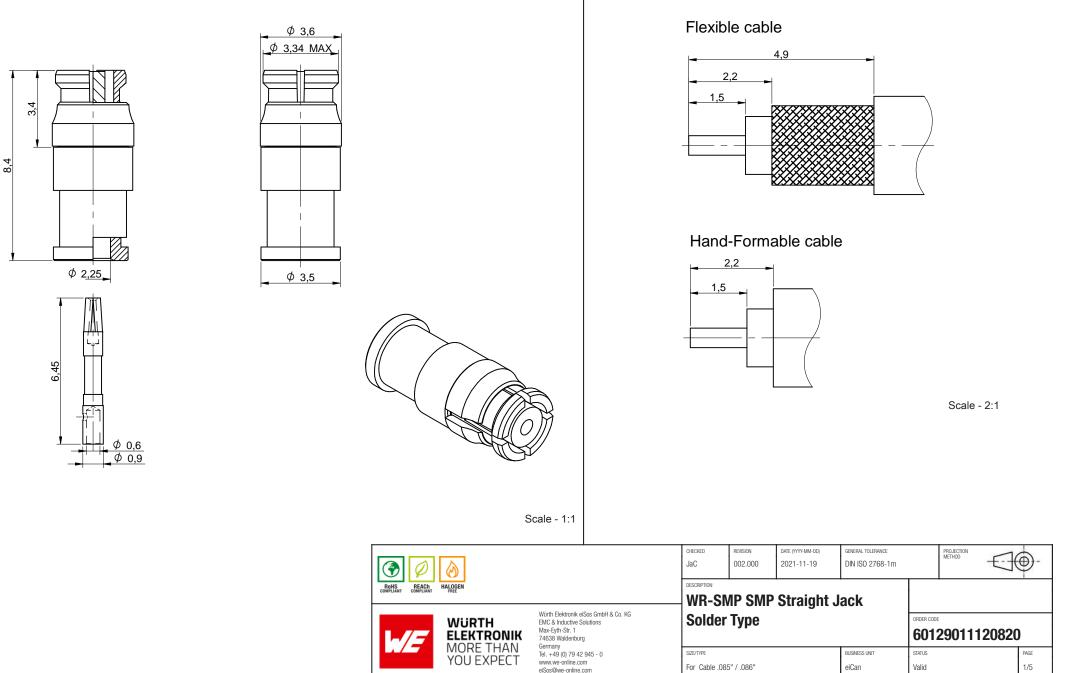
**Recommended Cable Stripping Dimension: [mm]**
