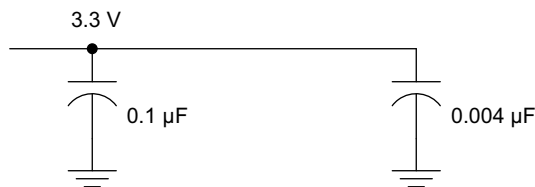
Figure 9-2. Recommended M-LVDS Bypass Capacitor Layout
