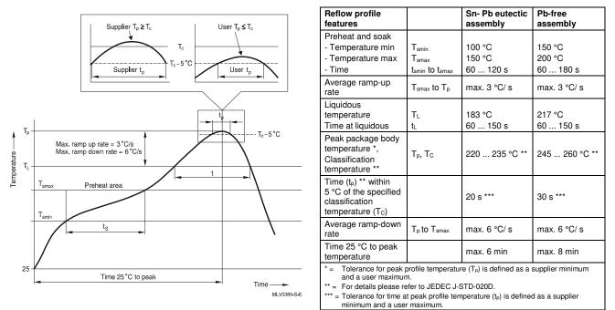
Surface mounted components (SMD) may exhibit a temporary increase in the DC spark-over voltage after the solder reflow process. The components will recover within 24 hours. There is no quality defect nor change in protection levels during the temporary change in DC spark-over voltage.
