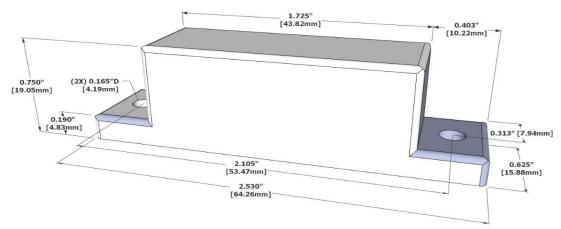
All measurements are in inches [millimeters]
