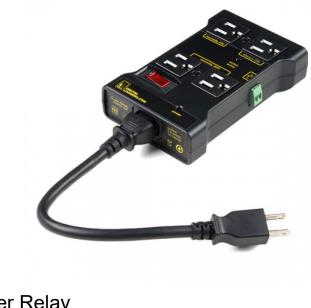
The IoT Power Relay is designed to allow you to safely control an outlet device that operates at 3--48VDC or 12--120VAC. Each IoT Power Relay features a single input (from the included C13 power cable) to four outputs: one normally on, one always on, and two normally off. The durable SPDT control relay is rated at 30/40A, for 400,000 operations.
