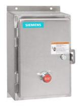
Non-reversing motor starter Size 0 Three phase full voltage Solid-state overload relay OLRelay amp range 0.75-3.4A 110VAC 50HZ / 120VAC 60HZ coil Combination type Water/dust tight non-corrosive
