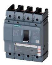
circuit breaker 3VA5 UL frame 250 breaking capacity class M 35kA @ 480V 4-pole, line protection TM230, FTAM, In=90A overload protection Ir=90A fixed short-circuit protection li=5...10 x In N conductor protection 100% without connection
