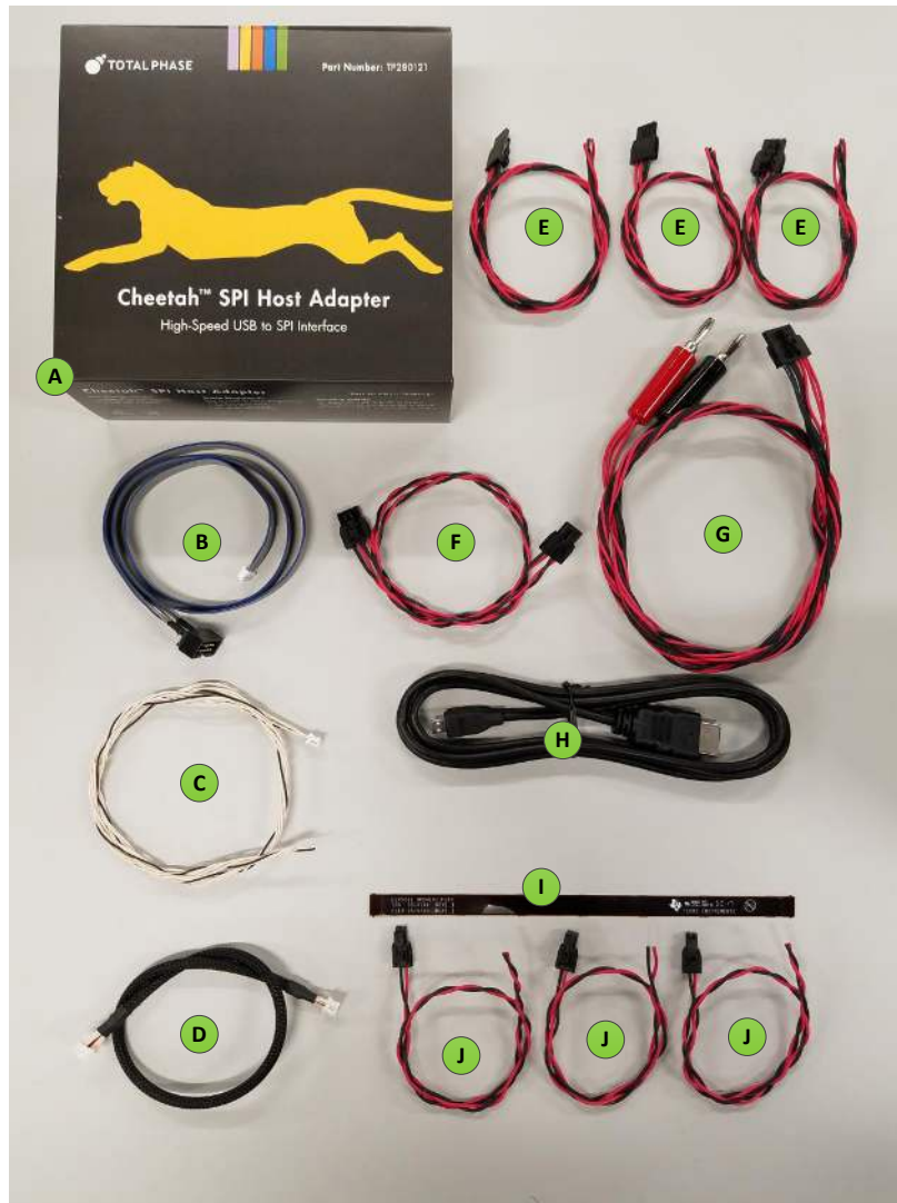
Figure 3. Cables Included in DLP5531-Q1 Light Engine EVM
