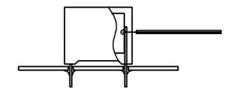
Temperature monitored inside the capacitor.
