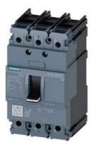
circuit breaker 3VA5 UL frame 125 breaking capacity class M 35kA @ 480 V 3-pole, line protection TM210, FTFM, In=90A overload protection Ir=90A fixed short-circuit protection Ii=10 x In UL489 SB (naval), 50 deg. cel. nut keeper kit on both sides
