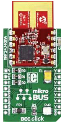
BEE Click Microchip's MRF24J-40MA 2.4 GHz IEEE 802.15.4 radio transceiver module.
