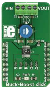
Buck-Boost Click Features LTC3129-1, a buck-boost DC/DC conversion integrated circuit.
