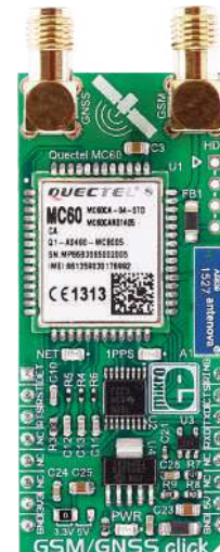
GSM/GNSS Click Quectel's MC60 quad-band GSM/GPRS/GNSS module. GPS/GNSS location tracking with GSM.
