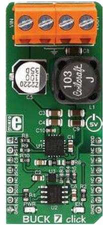
BUCK 7 Click The MAX17504, a high efficiency, synchronous step-down DC-DC converter with internal compensation.
