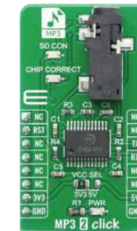
MP3 2 Click Based on KT403A, a hardware audio MP3/WAV decoder and DSP, with on-board microSD card slot.
