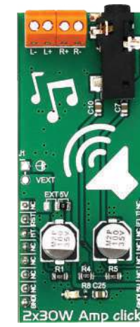
2x30W Amp Click The TPA3128, 2x30-W class-D amplifier with low idle power dissipation, from TI.
