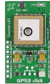
GPS3 Click With Quectel's L80, high-sensitivity GPS module with a patch antenna.
