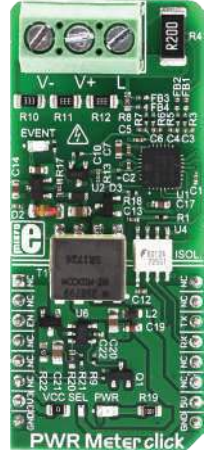
PWR Meter Click Uses the MCP39F511A, a very sophisticated monitoring IC from Microchip, with 16-bit processing core.
