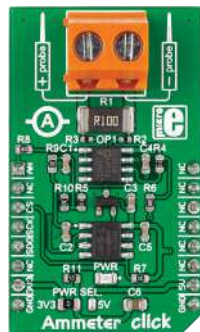
Ammeter Click With circuitry for measuring electric current (AC and DC). 0.1A-1A measurement range.
