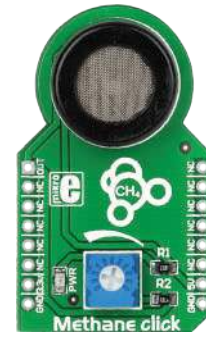
Methane Click With MQ-4 sensor for methane [CH 4 ]. Detection range 200-10000ppm of CH 4 .
