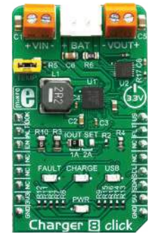
Charger 8 Click The MAX8903B and the MAX17201, both ICs from Maxim Integrated.
