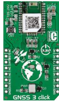
GNSS 3 Click Carries SIM33ELAGNSS module with an integrated antenna and an external antenna connector.
