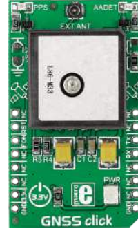
GNSS Click Quectel's L86 GNSS module with a patch antenna and an external antenna connector.
