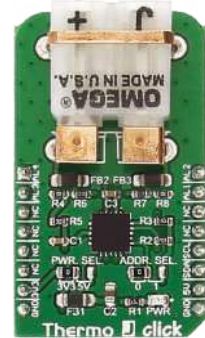
Thermo J Click It is a temperature measurement Click board™, which uses a thermocouple type-J probe. MSRP - $24 00 MIKROE-2811
