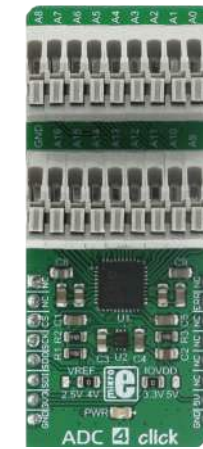
ADC 4 Click An advanced analog to digital multichannel converter. It can work in 16bit or 24bit mode.
