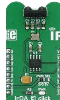
IrDA 3 Click Intelligent IR transceiver device that sends and receives UART commands via the IRT interface. MSRP - $26 00 MIKROE-2871
