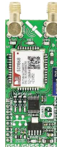
GSM/GNSS 2 Click With SIM868 quad-band GSM/GPRS module. GPS/GNSS location tracking with GSM.
