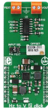
Hz to V 2 Click With the VFC32KU, a voltage-to-frequency and frequency-to-voltage converter.
