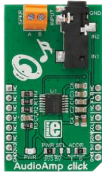
Audio Amp Click A mono audio amplifier. With TI's LM48100Q-Q1 Boomer™ Mono, 1.3W Audio Power Amplifier IC.
