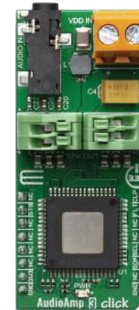
Audio Amp 3 Click Based on the Si4731 IC - digital CMOS AM/FM radio receiver from Silicon Labs.
