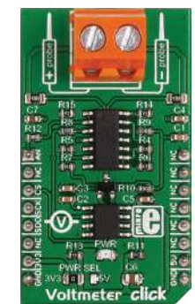
Voltmeter Click For measuring voltage in an external electric circuit. Measures direct current [from 0 to 24V].
