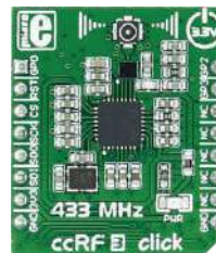
ccRF 3 Click Carries the CC1120 high-performance RF transceiver for narrow-band systems from TI.
