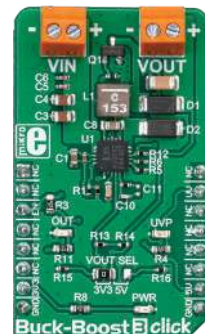
Buck-Boost 3 Click The ISL85403, a 2.5A regulator with the integrated high-side MOSFET and a low-side driver.
