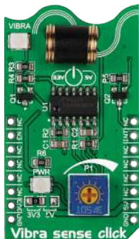
Vibra sense Click A micro shock vibration sensor with a digital output. For anti-tampering, anti-theft devices. MSRP - $18 00 MIKROE-1927
