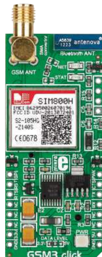
GSM 3 Click With SIM800H quad-band GSM/GPRS module. 85.6 kbps GPRS data transfer.
