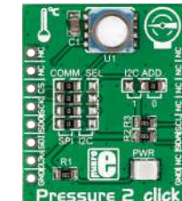
Pressure 2 Click With MS5803, a high resolution MEMS pressure sensor. Range 0-14 bars, resolution up to 0.2 mbars.
