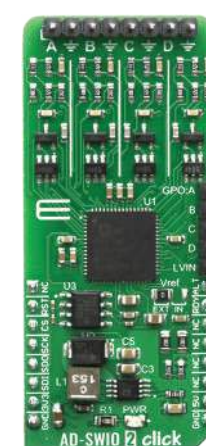
AD-SWIO 2 Click With a 16-bit ADC converter, and 13-bit DAC converter integrated into the AD74413R.
