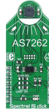
Spectral 2 Click Uses the AS7262, 6 channel visible spectral_ID device with electronic shutter and smart Interface.
