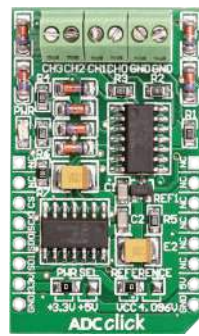
ADC Click With Microchip's MCP3204 12-bit Analog-to-Digital converter.
