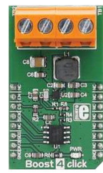
Boost 4 Click Carries TI's TPS61230A, a high efficiency fully integrated synchronous boost converter.
