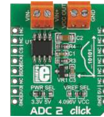
ADC 2 Click With MCP3551/3, a 22-bit ADC with automatic internal offset and gain calibration.
