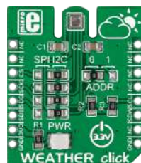
Weather Click With BME280 integrated environmental unit. Detects humidity, pressure, and temperature. MSRP - $22 00 MIKROE-1978
