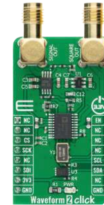
Waveform 2 Click Features the AD9834, a 75 MHz low power DDS device.
