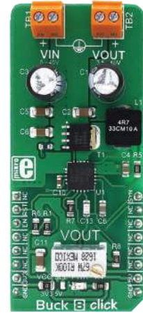
Buck 8 Click Uses the MAX17536, a high-efficiency, synchronous step-down DC-DC converter.
