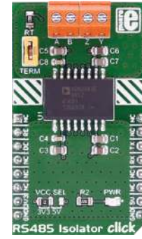
RS485 Isolator Click With ADM2682EBRIZ, a 5 kV RMS signal and power isolated RS-485 transceiver. MSRP - $49 00 MIKROE-2673
