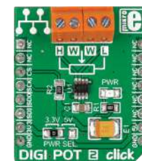
DIGI POT 2 Click Carries a single channel digital potentiometer TPL0501 with 256 wiper positions.
