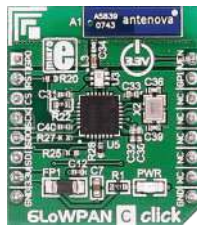
6LoWPAN C Click TI's CC2520, 2.4GHz ZigBee®/IEEE 802.15.4 RF transceiver.
