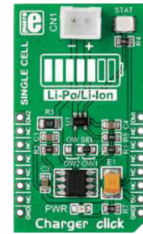
Charger Click Carries a battery charger controller and a battery charge monitor, along with a battery connector.
