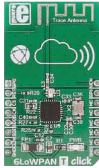
6LoWPAN T Click TI's CC2520, 2.4GHz ZigBee®/IEEE 802.15. RF transceiver.
