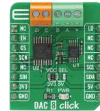
DAC 8 Click The DAC8554IPWR, a 16-bit QUAD channel voltage-output digital to analog converter.
