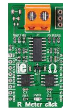
R Meter Click With circuitry for measuring the value of resistors. A wide range of resistors [0-1 Mega Ohm].
