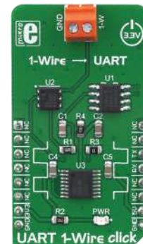
UART 1-Wire Click Designed to convert standard UART or RS232 signals into 1-Wire® signals. MSRP - $22 00 MIKROE-3340
