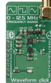
Waveform Click The AD9833, a low-power, programmable waveform generator.
