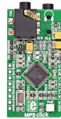
MP3 Click With a stereo MP3 decoder VS1053. Multiple formats (MP3, MP1, MP2, MPEG4, etc.).
