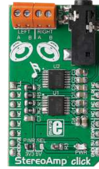
StereoAmp Click With 2 TI's LM48100Q-Q1 Boomer™ single supply, mono, bridge-tied load amplifier ICs.
