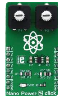
Nano Power 2 Click The MAX40000AUT12+, a nanoPower comparator with built-in reference.
