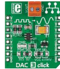
DAC 3 Click Carries Microchip's MCP4726 IC, a 12-bit digital-to-analog converter.
