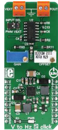
V to Hz 2 Click With the VFC32KU, a voltage-to-frequency and frequency-to-voltage converter.
