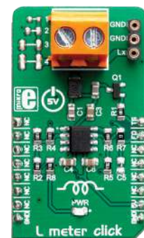
L meter click Features the LM311D, a high-speed voltage comparator.
