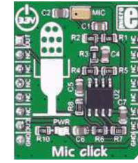
Mic Click With SPQ0410HR5H-B surface mount silicon microphone with max. RF protection.
