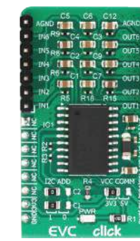
EVC Click The PT2258, a six-channel electronic volume controller IC, from Princeton Technology Corp.
