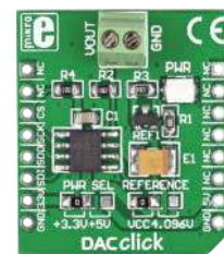
DAC Click Includes a 12-bit Digital-to-Analog Converter MCP4921 from Microchip.
