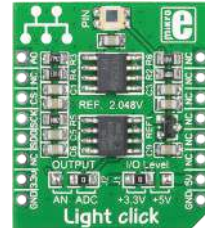
Light Click Used to measure ambient light intensity, with PD15-22CTR8 PIN photodiode.
