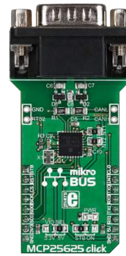
MCP25625 Click With CAN control-ler with an integrated transceiver. High speed operation up to 1 Mb/s. MSRP - $24 00 MIKROE-2228
