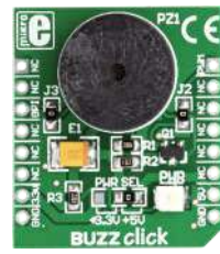
BUZZ Click Features a piezo speaker capable of emitting audio signals. Resonant frequency 3.8 kHz.
