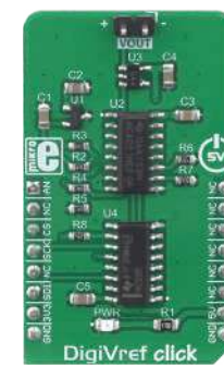
DigiVref Click With the MCP1541 it is a perfect solution to be used in various A/D conversion applications.
