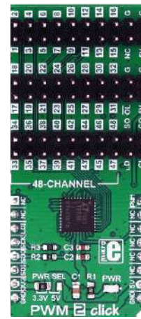
PWM 2 Click With the LT8500, a 48-Channel LED PWM generator with 12-Bit res. and 50MHz serial interface. MSRP - $19 00 MIKROE-3148
