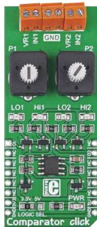
Comparator Click Carries LM2903 IC, has two independent precision voltage comparators. 2 mV offset voltage.
