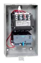
Non-reversing motor starter Size 00 Three phase full voltage Solid-state overload relay OLRelay amp range 0.25-1A 220-240/440-480VAC 60HZ coil Combination type Indoor general purpose use
