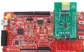
Fig 4: Programming and debugging with CY8CKIT-042-BLE Pioneer Kit Baseboard
