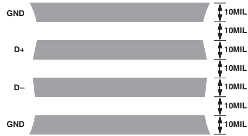
Figure 4. Arrangement of Signal Tracks
