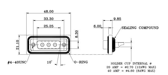
NOTE: MATERIAL HOUSING PBT UL94V-0, BLACK FLANGE PBT UL94V-0, BLACK CONTACT BRASS, PLATING P/N KEY BELOW SHELL STEEL, NICKEL O-RING SILICONE **EPOXY** SEALING COMPOUND HARDWARE BRASS; NICKEL PLATED ELECTRICAL POWER CONTACT RATED CURRENT P/N KEY BELOW VOLTAGE 1000 VAC 1 MIN INSULATOR RESISTANCE 5 G0hms MIN. POWER CONTACT RESISTANCE 2.0 m0hms MAX. WATER PROOF **IP67** ENVIRONMENT
