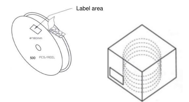
According to MSL1 packing requirement, MBB-Moisture Barrel Bag, Desiccant, HIC-Humidity Indicator Card, MSID Label, Caution Label are required.
