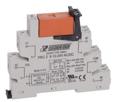
Plug-Relay-Compact (PRC) socket base PRC with screw connection, Mounting type: Mounting rail TS 35, 2 CO contact, Input voltage: 6.12 or 24 VAC/DC
