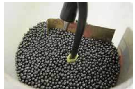
Figure 6 - Dielectric Strength Test - PLASTI-GRIP Terminal
