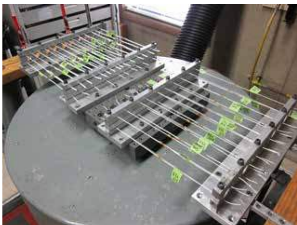
Figure 2 – Military Vibration Test - SOLISTRAND Splices
