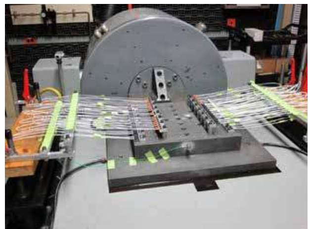
Figure 3 – Military Vibration Test - PIDG Terminals
