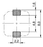
no sensitive traces underneath the component
