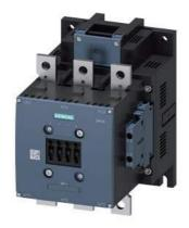
power contactor, AC-3 225 A, 110 kW / 400 V AC (50-60 Hz) / DC operation 42-48 V AC/DC auxiliary contacts 2 NO + 2 NC 3-pole, frame size S10 busbar connections drive: conventional screw terminal
