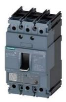
circuit breaker 3VA5 UL frame 125 3-pole, starter protection TM120M, AM, In=30A without overload protection short-circuit protection li=5...12 x In nut keeper kit on both sides
