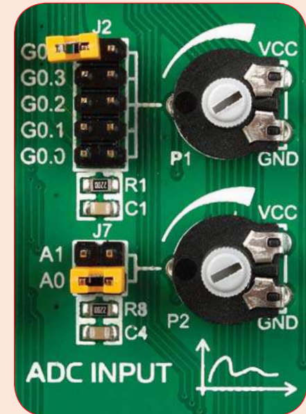
Figure 14-1: use J2 and J7 jumpers to connect analog input lines with potentiometers P1 and P2
