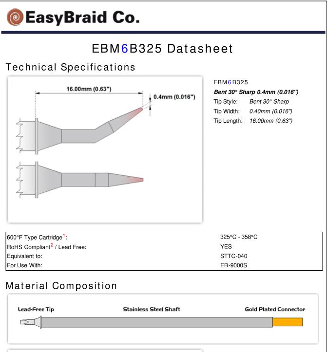
Copper Core Solder Iron Plating Copper Core Solder Iron Plating 1 Easybraid tip cartridges will typically idle within a temperature range of +/-1.1°C. However, there is variation in idle temperature across tip geometries within an individual temperature series. Easybraid offers a wide variety of tip geometries from 0.4mm fine point tip to 5m chisel. The length and geometry of a tip will
