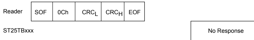
Figure 52. Reset_to_inventory frame exchange between reader and ST25TB02K
