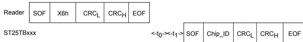
Figure 49. Slot_marker frame exchange between reader and ST25TB02K
