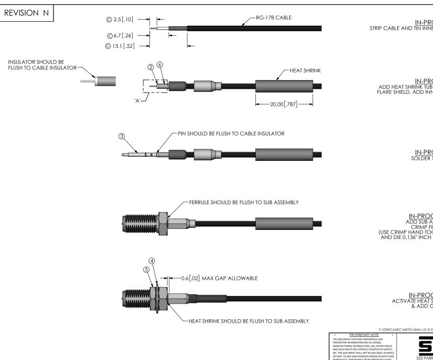
**IN-PROCESS 1** STRIP CABLE AND TIN INNER AND OUTER CONDUCTOR
