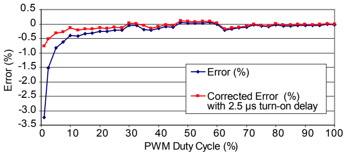
LED Current Error at 100 Hz PWM
