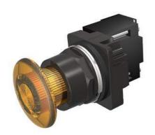
30mm BlackMax, Epoxy Coated Corrosion Resistant Complete Metal Unit Illuminated Push-Pull Operator Full Voltage, 24V AC/DC LED Lamp Mushroom Head Cap Small 1 3/4" (44.5 mm) Plastic, Amber 3 Position Pull-Momentary/Push-Maintained UL Listed, CSA Certified NEMA 1,3,3R,4,4X,12,13 & Automotive Standards
