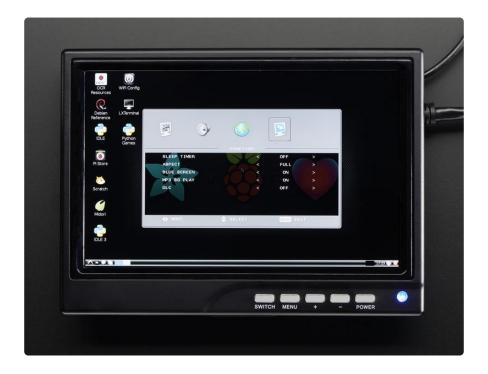
Sleep Timer - to 120 minutes - this will completely shut off the screen at the end of the set time  $\frac{1}{2}$
