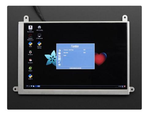
Power Saving - 10s to 60s - how long it takes for the screen to shut off Burnin - On/Off - a function to prevent screen burn-in ()
