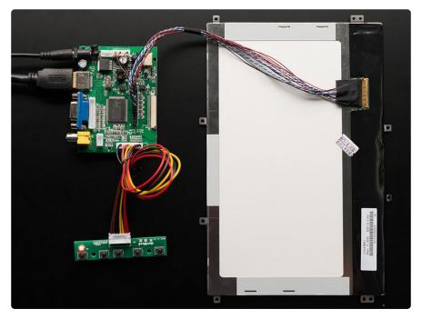
This is one of our prettiest display It's got excellent resolution (1280x800!) and IPS display so it is bright, crisp and looks good from any angle. This driver even has HDMI audio support and can drive two 4 ohm speakers directly.
